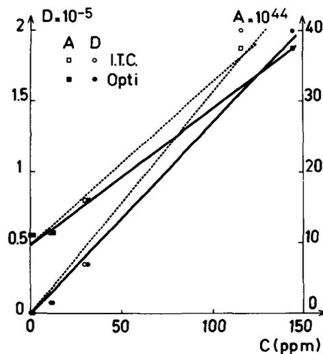
Fig. 5. — Plot of  $A$  (squares, scale on the right) and  $D$  (circles, scale on the left) coefficients vs. impurity concentration for KCl:Pb samples of figure 2. Open symbols: their abscissa is the concentration determined by I.T.C. measurements, i.e.  $n_{I.V.}$ ; Full symbols: their abscissa is concentration determined by optical absorption measurements, i.e.  $n_i$ .
