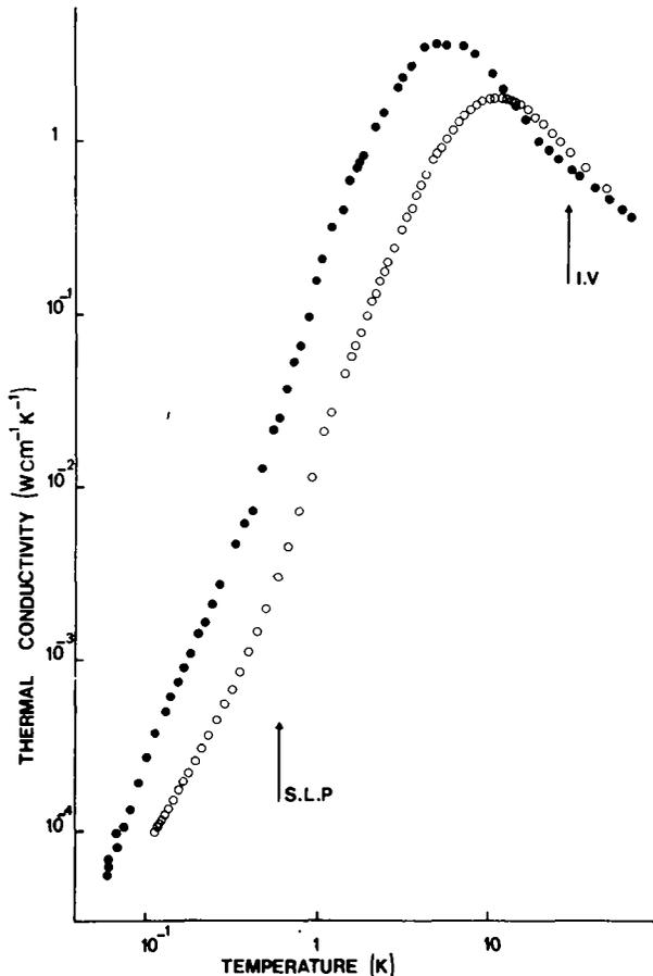
Fig. 1. — Thermal conductivity vs. temperature plot for KCl:Pb (32 ppm); full circles : sample quenched from 500 °C; open circles : 300<sup>h</sup> annealing.
