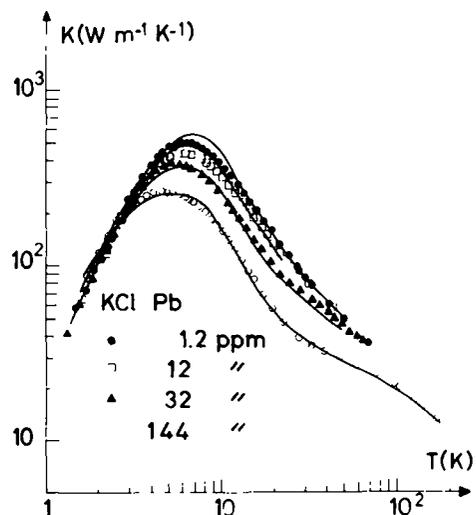
Fig. 2. — Thermal conductivity vs. temperature plot for KCl samples containing different Pb concentrations ( $n_t$ ), quenched from 500 °C. Circles, squares and triangles give the experimental points; the lines give the fitting.
